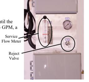
Run the system until the water turns clear, about 15 minutes. This will allow the feed water to flush out the RO system.
