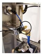
C. Run the remaining section of ½" blue hose from the already attached service fitting on the service flow meter (tag marked "D") to the site supplied drain.
